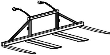
(useable fork length reduced by spreader tube size)
